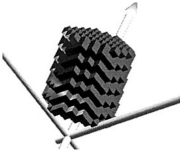
FIG. 7. The contact modeled as cylinder placed in a discrete (voxelized) space.
